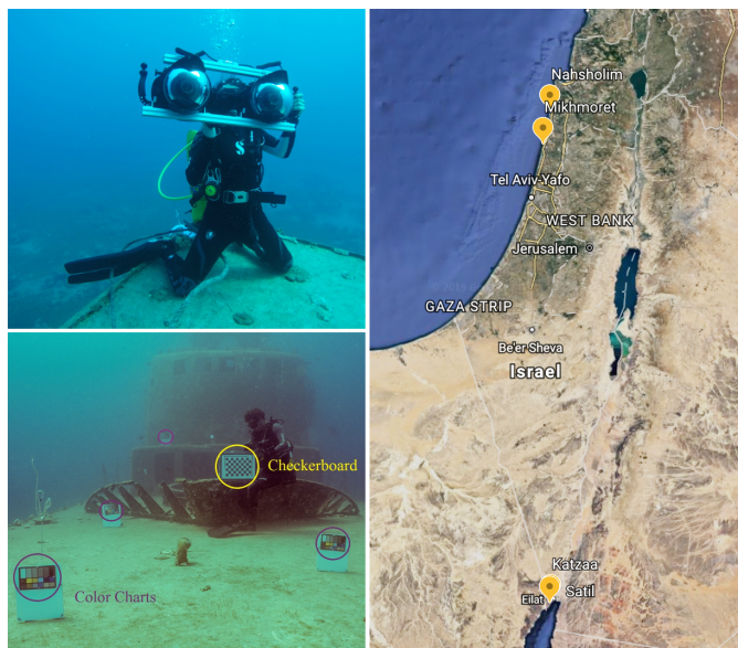
Fig. 5. Creating the dataset. [Top left] The stereo rig used for acquisition. [Bottom left] The color charts and calibration checkerboard. [Right] Dive sites' location.
